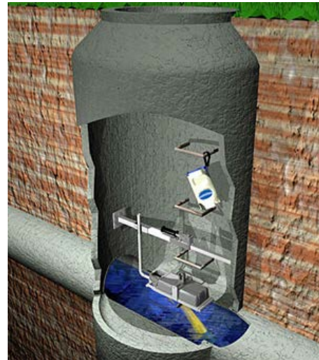
Figure 10. Typical Hach Marsh-McBirney Flo-Dar Installation
